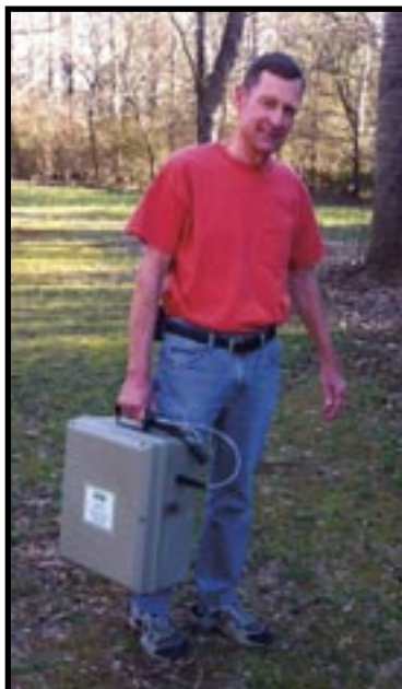
The compact self-contained Scout III weighs 19 pounds with empty sample container
